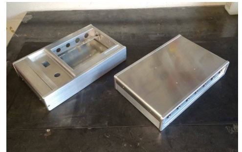
Control panel for an industrial laser-marking machine, fabricated from sheet metal and machined parts per customer drawings
