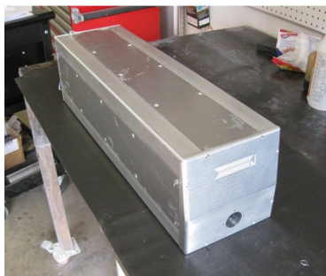
Enclosure for an industrial laser-marking system, machined from customer drawings
