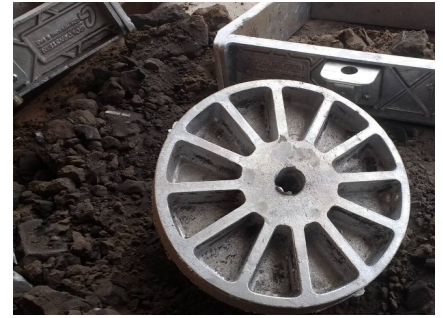
Prototype cast engine dynamometer water brake rotor
