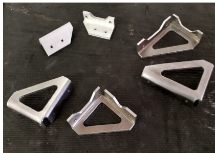
Prototype sheet metal parts to hold PCB in aerospace electronics enclosure
