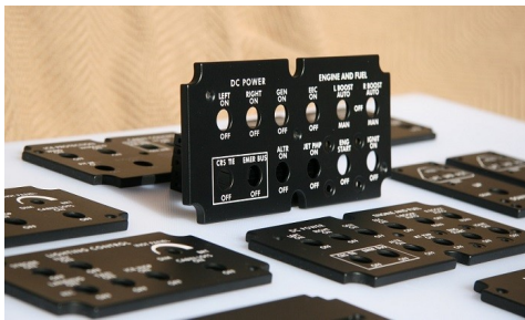
Aircraft cockpit back-lit panels — DC power & engine/fuel controls
