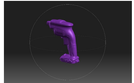
3D scan of power tool for reverse engineering
